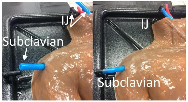
**4c.** Turn the pump on. Water should begin pouring out of the chest end of the vein in the trainer.
